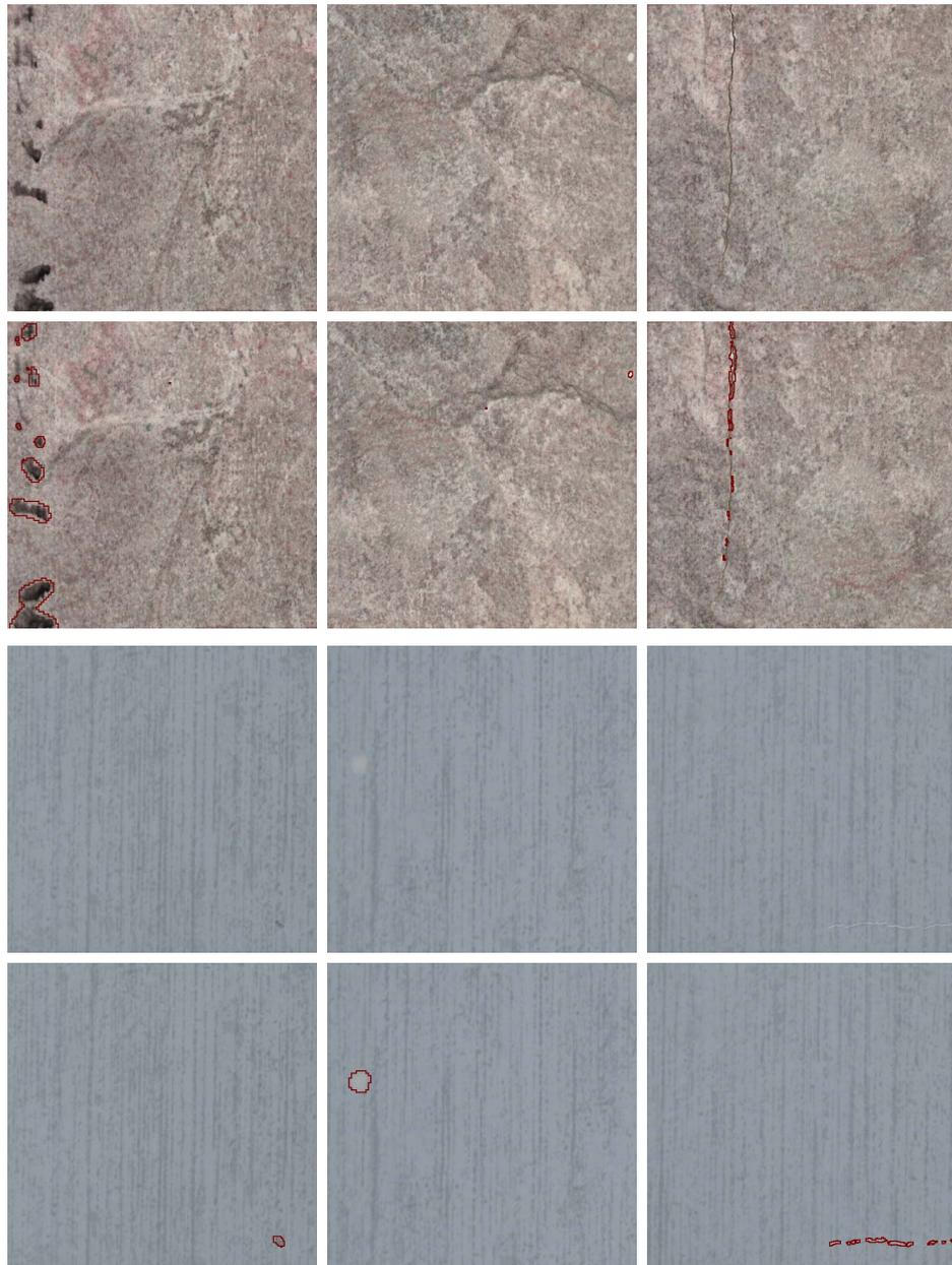
**Figure 6.6:** Defect localisation - The examples given in the top row are from the same tile family richly decorated with macro-structure patterns. Defects shown in the next row, from left to right, include print error, missing print, and thin surface crack. The next three images show a texture with oriented patterns. Defects shown in the last row, from left to right, include misprint, missing print, and subtle surface crack.
