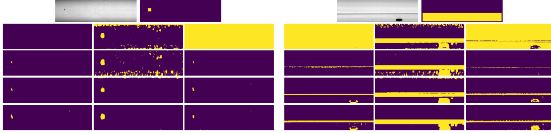
Figure 4.5: We show a forward pass of a single image of steel producing a dense segmentation over refinement sessions with three different experiments. This is accomplished via the graphical interface where the user is given the 5 worst negatives and positives based on an anchor, then selects new centre pixel for that patch. Row one displays the image and the initial ROI mask. Column one is based on user refinement, column two is mask updates, and column three is user refined with entropy anchor selection. Each row shows a subsequent refinement after a session.
