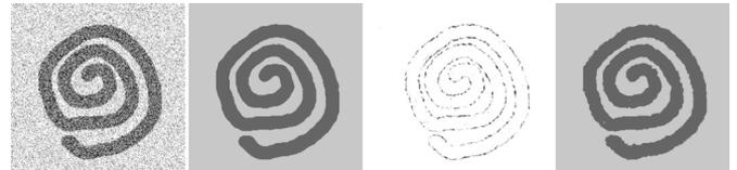
Fig. 12. From left: Complex shape with 50% Gaussian noise and the recovery result using force diffusion ( $K = 0.2$ ); heavily thresholded edge map with numerous broken and weak edges and its recovery result without force diffusion, i.e.,  $K = 0$ .
